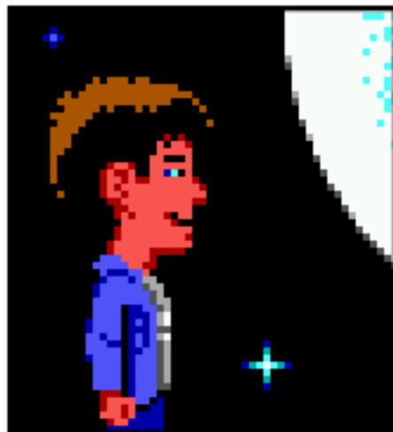
Fig. 3: 3x : No filtering, scales the image by a factor of 3.
