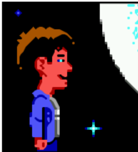
Fig. 10: HQ3x : Very nice high quality filter, but slow. Uses lookup tables to create anti-aliased output. Factor 3x.
