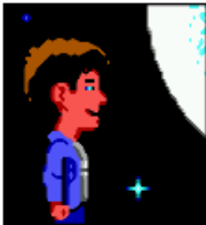
Fig. 5: Super2xSAI : Enhanced 2xSAI filtering, factor 2x.
