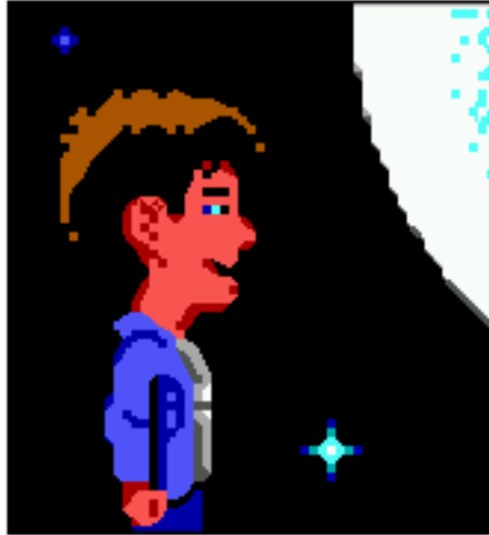
Fig. 8: AdvMAME3x : Doesn't rely on blurring like 2xSAI, fast. Factor 3x.
